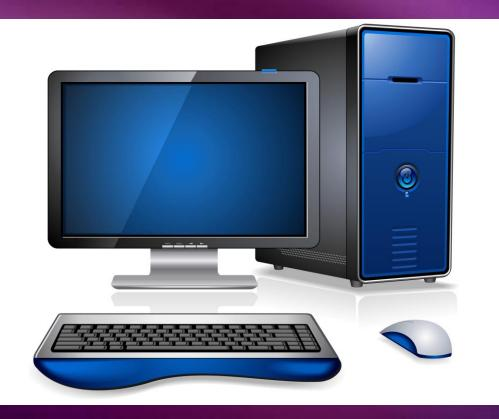
Computer hardware includes a central processing unit, input devices, output devices, and memory storage devices.
