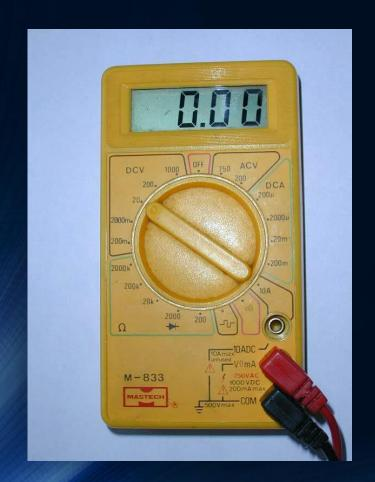
A device used to measure voltage, or electrical potential energy difference.
