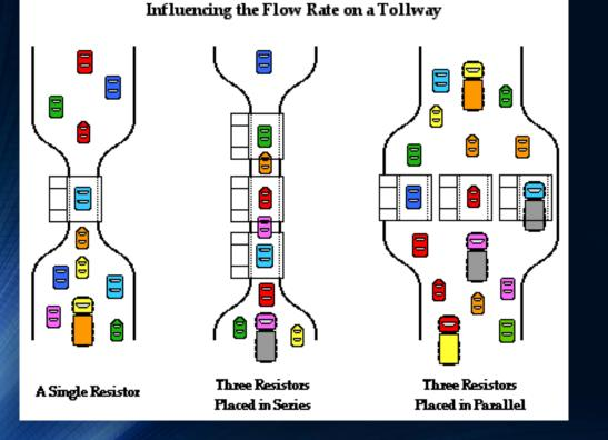
The greater the resistance, the less current there is for a given voltage.
