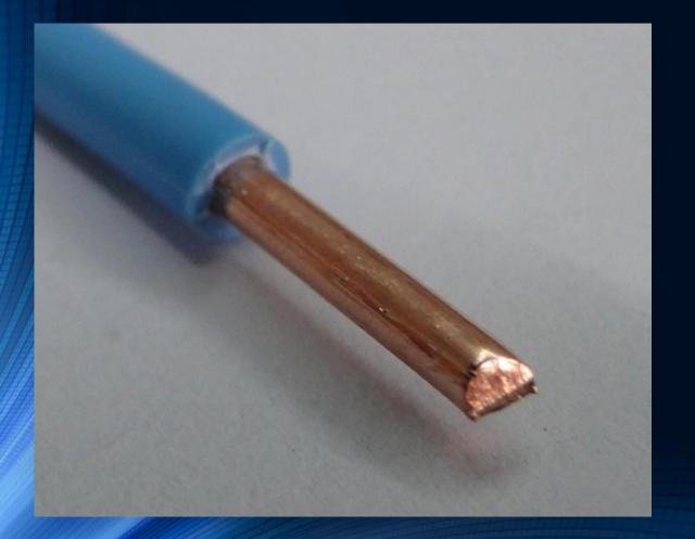
A conductor transfers electric charge well. An insulator does not transfer electric charge well.
