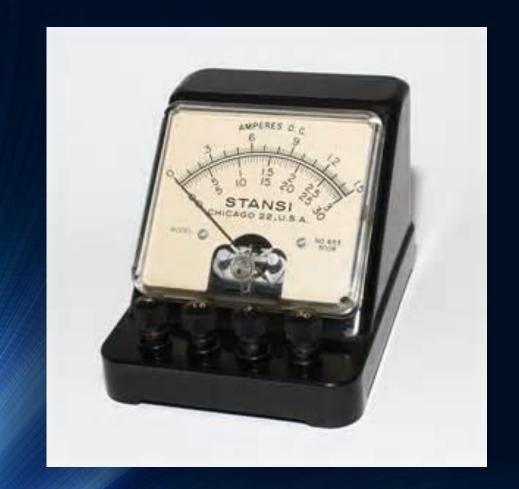
A device used to measure current in a circuit.
