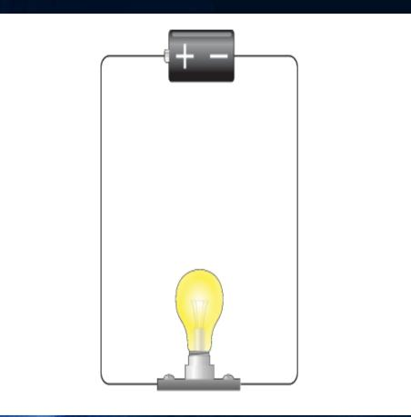
A complete, unbroken path through which electric charges can flow.
