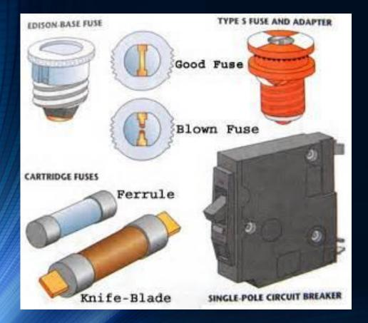
In order to prevent circuits from overheating, devices called fuses and circuit breakers are added to circuits.
