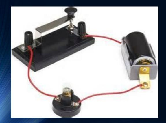
A device that creates an electrical potential energy difference in an electric circuit
