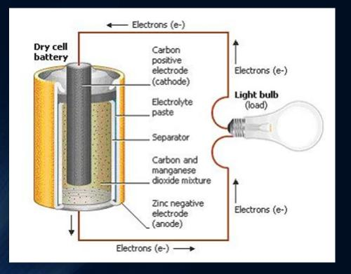
a metal part of an electrochemical cell which gains or loses electrons.
