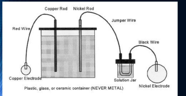
An electrochemical cell in which the electrolyte is a liquid.
